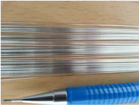
Nickel Micro Tube after removing SUS wire / 0.27φ
